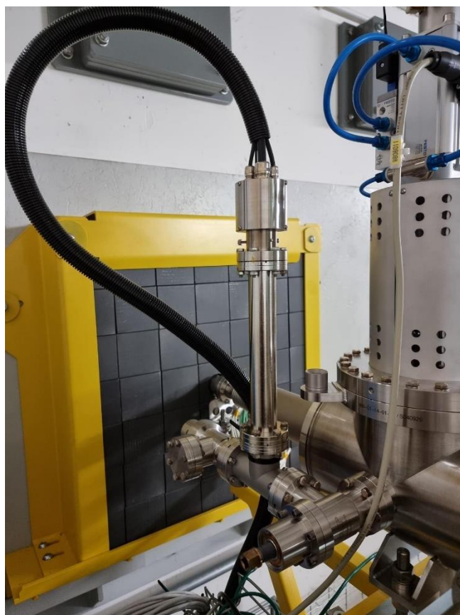
RGA HIDEN HAL 101 RC installed in the front-end vacuum chambers
