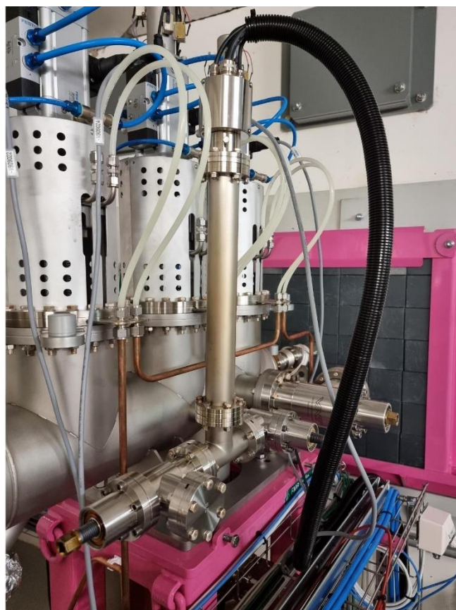
RGA HIDEN HAL 101 RC installed in the front-end vacuum chambers
